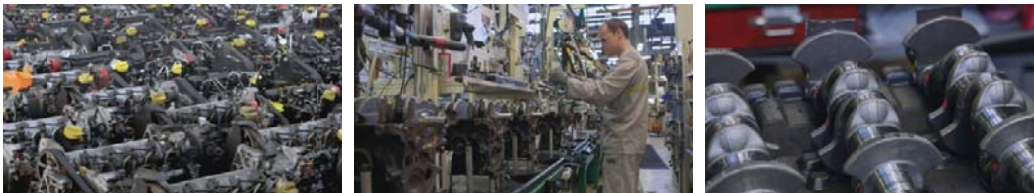
Reconditioning powertrain components from ELVs at Renault’s Choisy-le-Roi plant.
