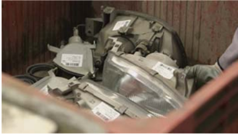
Sorting light units from ELVs for reuse at Indra’s Romorantin site
